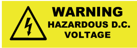
Example of sign on PV Array junction box (Clause 5.3.2)
