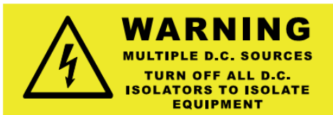
Example of sign required where multiple isolator / switch-disconnector devices are used (Clause 5.5.2)
