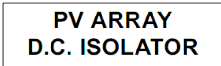
Example of sign required adjacent to PV Array DC isolator / switch-disconnector (Clause 5.5.2)
